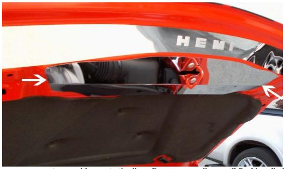
Your cover comes to you with a protective liner. Do not remove liner until final installation.
